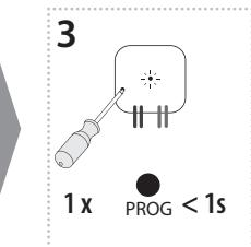
Press of programming button on receiver RFSA-62B shorter then 1 second will finish programming mode. The LED lights up according to the pre-set memory function.
