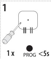
Press of programming button on receiver RFSA-62B for 3 - 5 second will activate receiver RFSA-62B into programming mode. LED is flashing in 1s interval.
