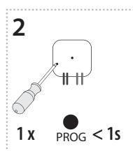
Pressing the programming button on the RFSA-62B receiver for less than 1 second will finish the programming mode, this will reverse the memory function. The LED lights up according to the current pre-set memory function. The set memory function is saved.
