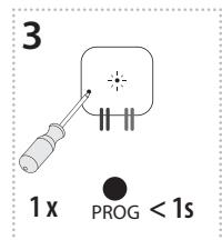
Press of programming button on receiver RFSA-62B shorter then 1 second will finish programming mode. The LED lights up according to the pre-set memory function.
