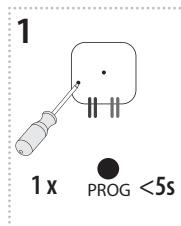
Press of programming button on receiver RFSA-62B for 3 - 5 second will activate receiver RFSA-62B into programming mode. LED is flashing in 1s interval.
