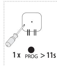
By pressing the programming button on the actuator for 11 seconds, deletion occurs of the actuator's entire memory. LED flashes 4x in each 1s interval. The actuator goes into the programming mode, the LED flashes in 0.5s intervals (max. 4 min.). You can return to the operating mode by pressing the Prog button for less than 1s. The LED lights up according to the pre-set memory function and the component returns to the operating mode. Deletion does not affect the pre-set memory function.
