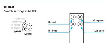
RF RGB mode for controlling RGB LED strips. In the RF RGB programming mode, colours are automatically assigned to individual transmitter buttons.
