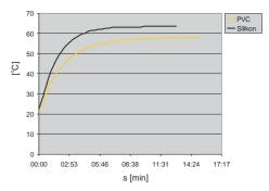
PVC -reaction to water temperature from 22.5 1°C to 58°C. Silicone - reaction to water temperature from 22.5°C to 63.5°C.
