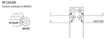
RF COLOR mode for controling RBG LED strips, where you can choose the color for individual transmitter buttons. A long press of the button starts the color search mode. After releasing the button, the current color is set for the given button Note: The mode can be controlled by iHC apllication, EST3, WSB3, GSB3, IM3 module and RFWB with RFIO2 protocol.
